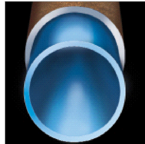
Shape of expanded pipe after being pressurized
