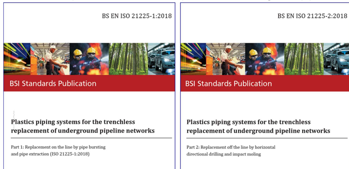
Fig. 4. EN ISO 21225 parts 1 and 2 covering the classification of four techniques for the trenchless replacement of underground pipelines
